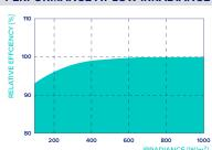
Typical module performance under low irradiance conditions in comparison to STC conditions ( $25\,^{\circ}\text{C}$ ,  $1000\,\text{W/m}^2$ ).
