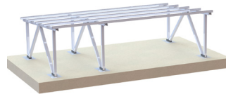
第三步 纵梁安装 Third Install the beam
