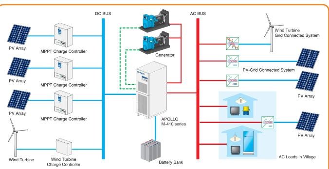
APOLLO M-410 series is a single phase bidirectional dual mode hybrid inverter capable of functioning as a main supply power source as well as providing automatic control and management of a generator and battery bank. The inverter features very high efficiency in both charger and inverter modes with maximum efficiency of 95%. It is suitable for hybrid power system with supplement diesel generator in off-grid areas.
