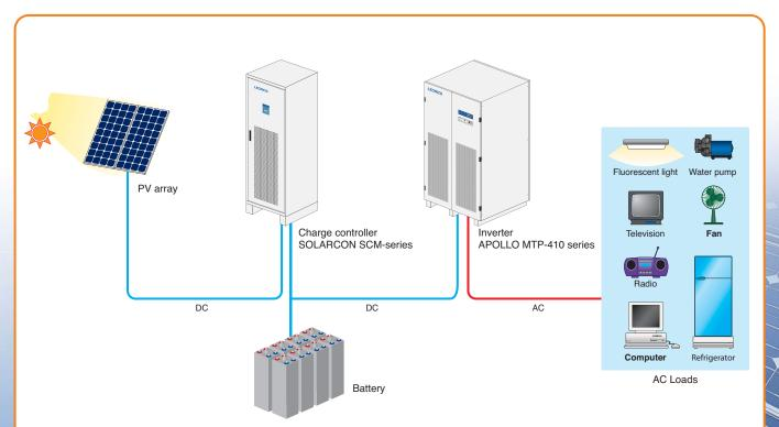
The SOLARCON SCM-series charge controller is the most sophisticate solar charger with PV Maximum Power Point Tracking (MPPT) algorithm. The charge controller equipped with advanced microprocessor control to get the maximum power from PV to charge battery with LCD display and front panel for easy and accurate setting more over the digital meter with 180 days power and event logger are inclusive
