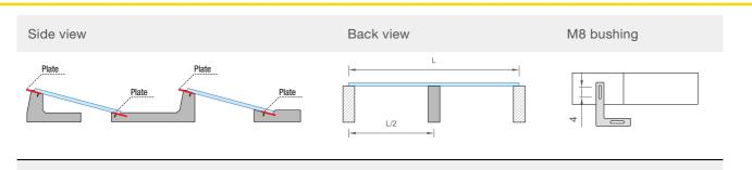
USE THE 4CM SLOT TO FIX THE PLATE ON THE CENTRAL REINFORCEMENT BALLASTS
