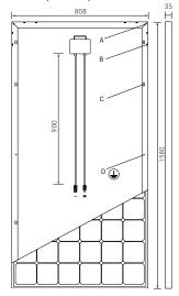
Drilled holes<sup>4</sup> A: 4 x drainage
