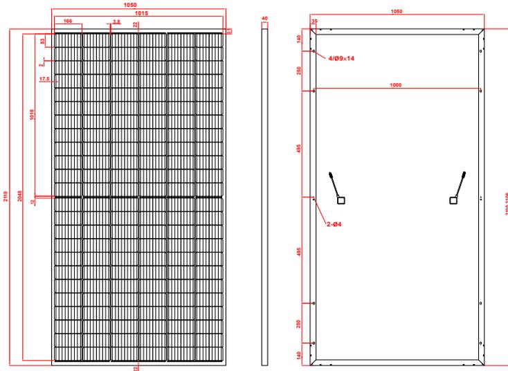
STC: Irradiance 1000 W/m<sup>2</sup>; Spectrum AM1.5; Cell Temperature 25°C, Wind 0 m/s
