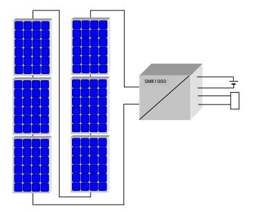
Configuration with maximum Solar voltage 6 modules - string, 216 cells. Cells.
