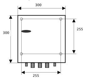
Height=150mm Mounting holes in bottom of housing D=10mm
