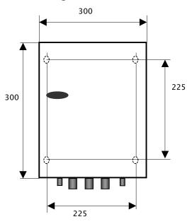
Height=150mm Mounting holes in bottom of housing D=10mm
