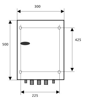
Height=210mm Mounting holes in bottom of housing  $D=10mm_{\underline{}}$
