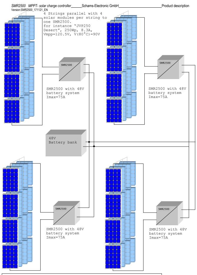
Total solarpower 16kWp. Total battery charging current 300A. Battery system voltage 48V.
