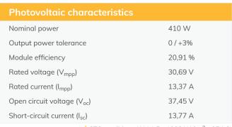
STC conditions (AM 1.5 - 1000 W / m<sup>2</sup> - 25 ° C) Measurement tolerance: +/- 3%
