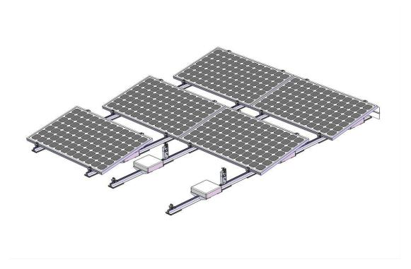
Powerack East & West Ballasted-B Is to be fixed anywhere on the long side. Therefore, solar panels could withstand greater wind and snow pressure. There is no need to use expansion bolts or chemical bolts on the roof, no damage to roof. The system connects all the panels with the rails into a whole. East-west facing panels have a great effect on resisting wind loads. A combination of high quality aluminium components make a robust, reliable system and quick and easy installation.
