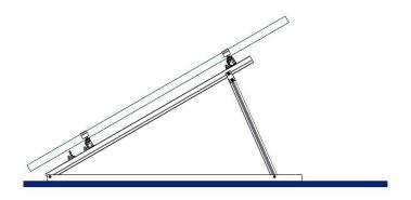
Mini Rail with 5 degree support base, lift up the height of the solar panel to achieve cooling conditions, thus maximizing power generation. Simple design, easy to install, with good price.
