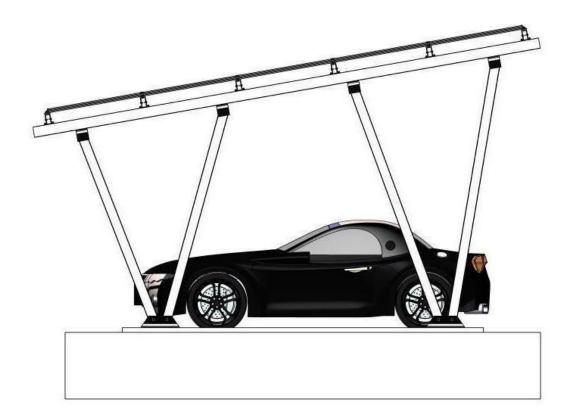
The carport solar mounting system provide power for electric vehicles and home. It can be used in homes, commercial areas and other outdoor places. It is stored in the battery via a charging unit or provided directly to the electric vehicle for self-consumption. You can even use the extra power to access the Internet. The system includes adjustable mounting brackets for easy installation on any surface. The components of the system are installed in advance, which saves time and labor.
