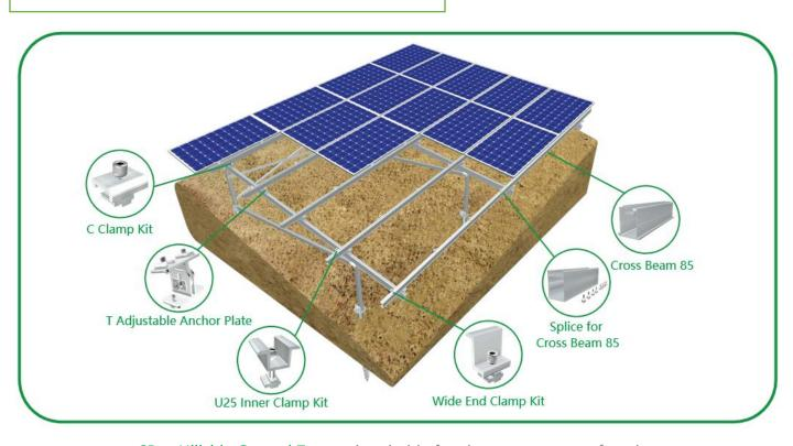
SRac Hillside Ground Terrace is suitable for slope concrete roof or slope land solar PV projects, with strong wind load and snow load resistance. The system can achieve minor adjustment onsite with special design of Anchor Plate to adapt to different sites. The system can be adjusted from eastwest and south-north direction with special connector design. Patented and certified system design ensure project's safety and quick installation.
