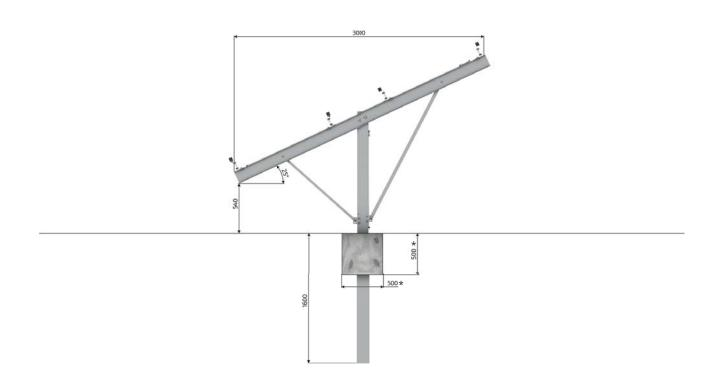
\* One of the possible variants of concrete casting. The concreting volume is determined by the design.
