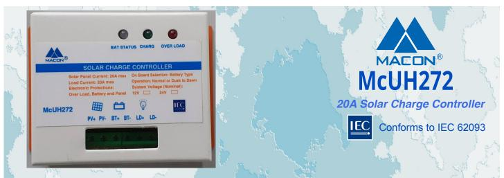
McUH272 is another quality Solar Charge Controller with 20A current capacity for load as well as for charging the battery. It is available in two versions, 12V nominal or 24V nominal. The same controller can be used for different type of batteries by selection on board. The controller can be used for normal and dusk to dawn operation simply by selection on board.
