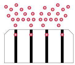
The soul of solar panels is the number and quality of the cell and the solder between them. Thus, the Hero series is made of the best "A" quality cell and 9 guidewires. Over the long years, it matters a lot if even 1 in 4 to 6 conductors detaches from the cell surface because the energy produced cannot pass through. In the case of 9 guide wires, this is not possible!
