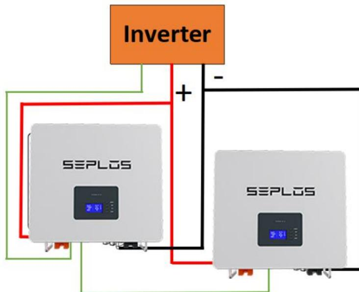
Scheme two : High power (multiple machines in parallel)
