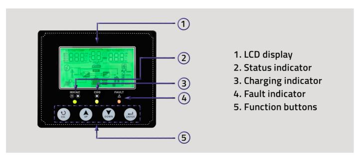
The product is equipped with a multifunctional, easy-to-use LCD display with control panel. Facilitates monitoring of the entire photovoltaic installation. Allows you to configure the input voltage range for home appliances and personal computers or change the priority settings of the AC/Solar charger. In addition, the display records data and informs about failures, reacting accordingly if any of the parameters exceed the norm. If a fault occurs, the inverter shuts down.
