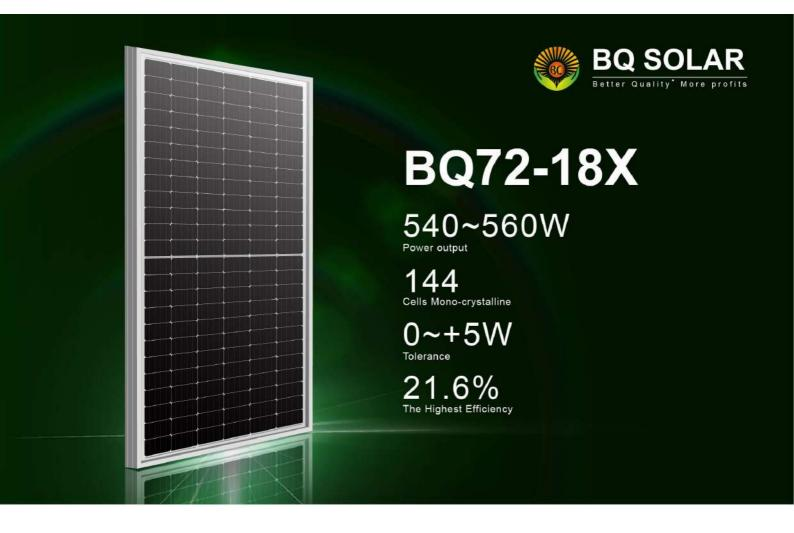
BQ18X HALF-CELL series is produced with high efficiency multi-busbar cells, which can reduce the module internal power loss to improve its conversion efficiency, as well as lower the failure risk caused by cracks and broken busbar to enhance the module reliability Combined with half-cell technology, the module is highly resistant to hot-spot crisis caused by shadow effect.
