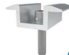
Middle Clamp Kit 30/35/40mm AL6005-T5&SUS304 Black optional
