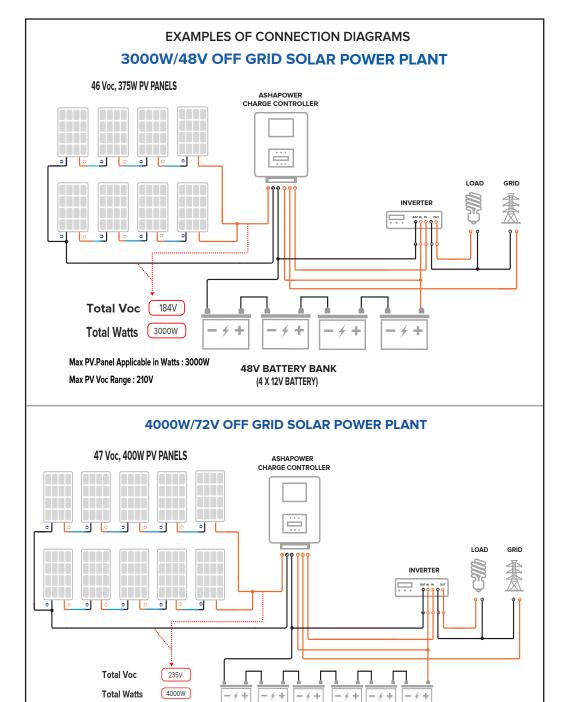
Max PV.Panel Applicable in Watts: 4000W
