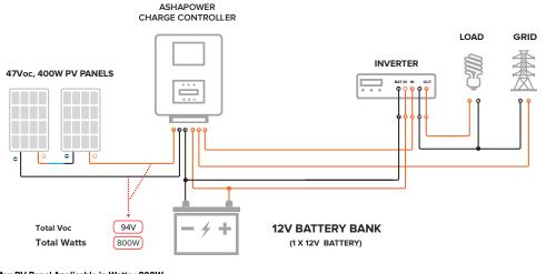
Max PV.Panel Applicable in Watts: 800W
