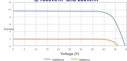
REAR SIDE IV CURVE @ 1000W/m 2 and 200W/m 2
