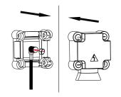
Note: Press the position indicated in the figure above before disconnecting the power terminal.
