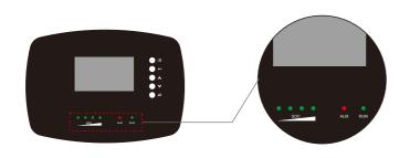
The BMS features 6 external LED indicator lights. 1. 4 white-green capacity indicator lights. 2. 1 red alarm indicator light. 3. 1 withe-green operational indicator
