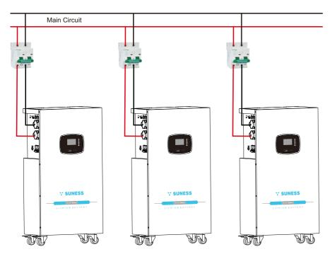
Step 1: The parallel connection of three battery packs is presented in Figure 1.
