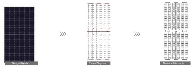
Module current output is 4.5+4.35=8.85A, current mismatch in series is **0.15A**.
