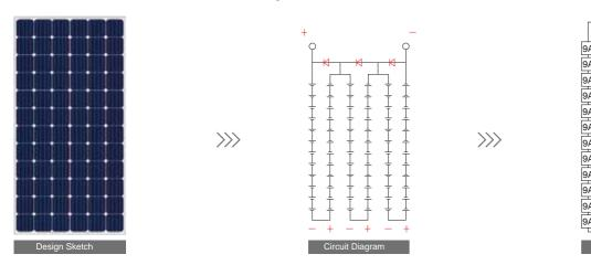
Module current output is 8.7A, current mismatch in series is **0.3A**.
