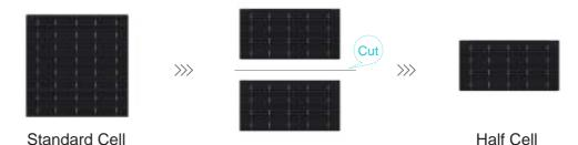
The ribbon length of half-cell is shorter than normal cell. Calculated by Joule's law and Ohm' law, the power loss reduction is nearly 6%.
