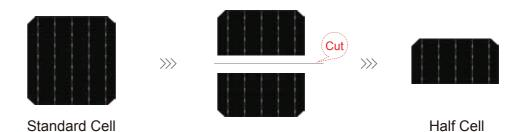
The ribbon length of half-cell is shorter than normal cell. Calculated by Joule's law and Ohm' law, the power loss reduction is nearly 6%.
