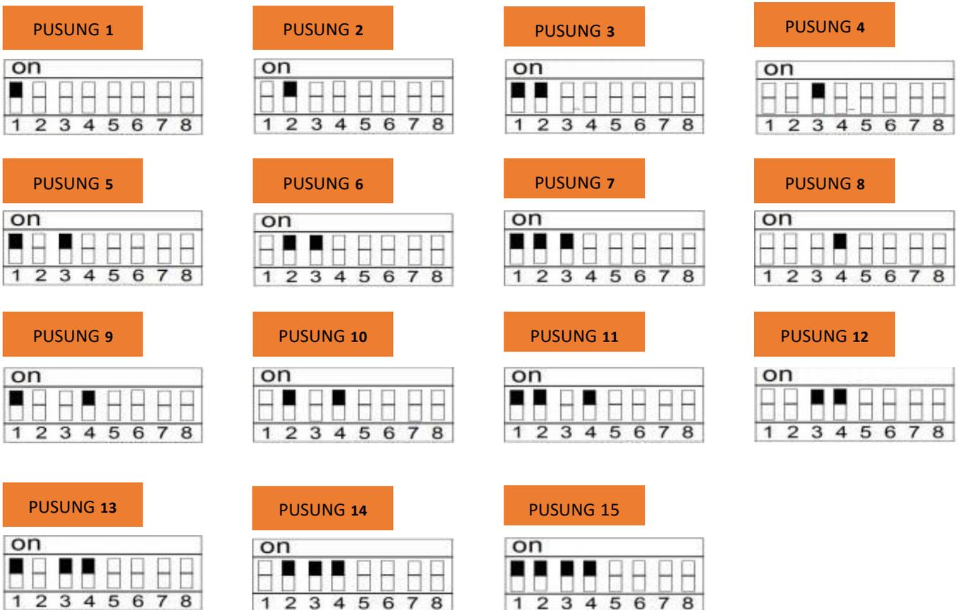
5.2 CAN BUS DIP address setup demonstration.
