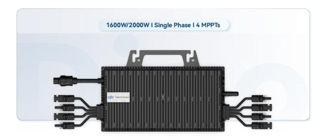
TBB DG1600/2000 microinverter is designed for residential on-grid PV systems and features 4 MPPTs, supporting 4 PV modules each. This allows for independent tracking of each module, and maintaining maximum power output even if a module is shaded or fails. The DG1600/2000 operates at lower voltages, reducing high voltage risks and enhancing safety.
