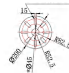
Size of the hole 15x45mm
