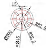
Size of the hole 15x45mm
