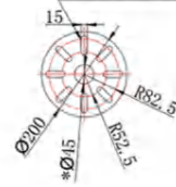
Size of the hole 15x45mm
