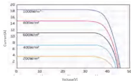
I-V/P-V Curve at Different Irradiation (655W)
