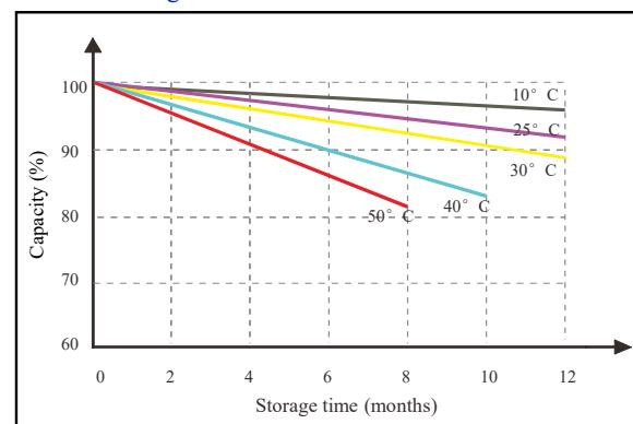
Note 2: The above curves are based on laboratory testing data @ 25°C 40%RH.
