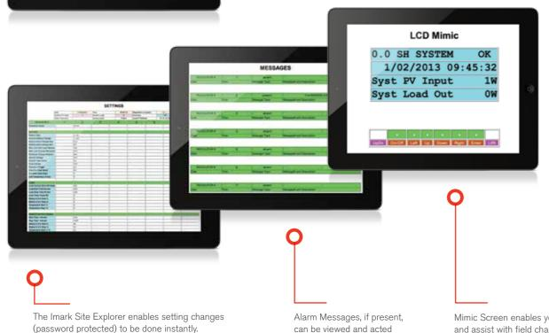
The Settings screen displays the settings for up to eight regulators in columns enabling easy settings comparisons or changes.
