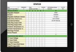
Monitor your system operation from anywhere using the Internet, or directly using a laptop, or PC. Regulator performance is updated at 15 second
