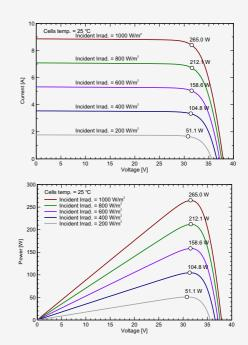
STC: Irradiance 1000W/m<sup>2</sup>,Module temperature 25°C,AM1.5 spectrum.
