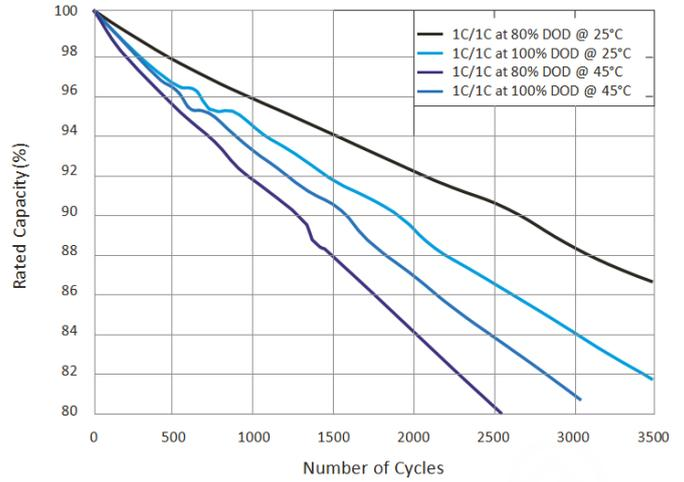
**1C Cycle Curves at Different DOD & Temperatures**
