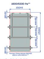
\*When a module is installed in portrait orientation on the pitched roof which as >45° slope, additional hook in the bottom of the module is required \*\*\*\*For details please refer to SoliTek SOLID installation manual 1013±5 1013±5
