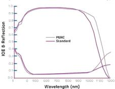
PERC technology enables better light capturing abilities at longer wavelength, weak and diffused light and in cloudy conditions.
