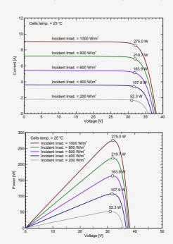
STC: Irradiance 1000W/m<sup>2</sup>,Module temperature 25°C,AM1.5 spectrum.
