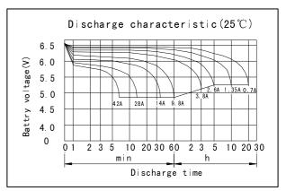
Rechargeable Valve Regulated lead-Acid Battery
