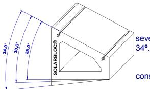
The Solarbloc® supports are manufactured in seven different grades, 10°, 12°, 15°, 18°, 28°, 30° and 24°
