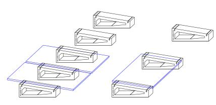
Solarbloc® with 10°, 12°, 15° and 18° allow mounting panels vertically and horizontally.
