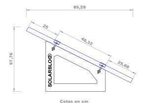
3- Finally, place the next panel and tighten the anchors to secure them.
