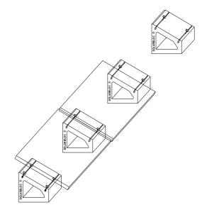
Each support includes two anchors required for fixing panels.
