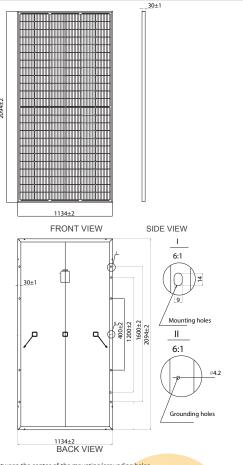
$<sup>\</sup>ensuremath{^{\star}}$  The distance between the center of the mounting/grounding holes.
