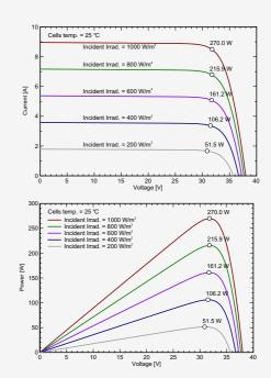
STC: Irradiance 1000W/m<sup>2</sup>,Module temperature 25°C,AM1.5 spectrum.
