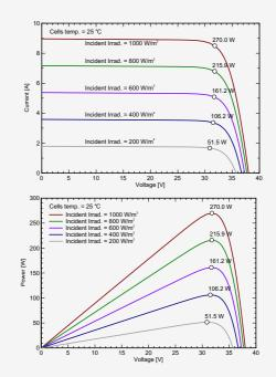
STC: Irradiance 1000W/m<sup>2</sup>,Module temperature 25°C,AM1.5 spectrum.
