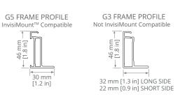
G5 frames have no mounting holes. Please read the safety and installation guide.
