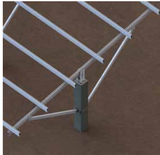
Square PHC Pile Structure Type I
