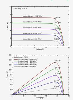
STC: Irradiance 1000W/m<sup>2</sup>, Module temperature 25°C, AM1.5 spectrum.
