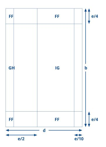
The required values for determining the ballast calculation for the roof areas. H and I as well as F and G must be calculated in accordance with the actual location.
