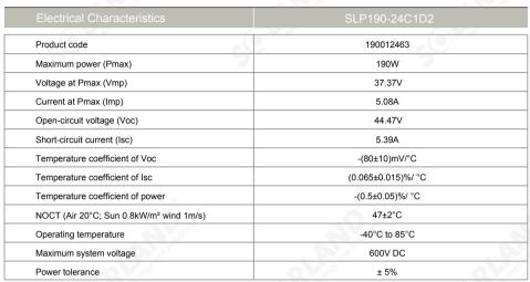
\*STC: Irradiance 1000W/m², AM1.5 spectrum, module temperature 25°C \*NOCT:Nominal operating cell temperature (the data is only for reference)
